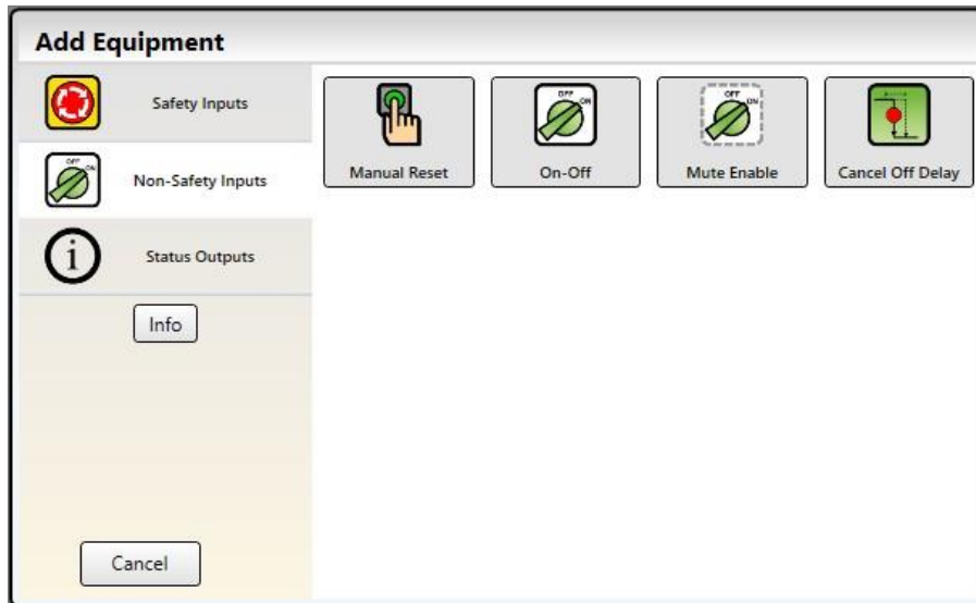
Figure 33: Non-Safety Inputs (Virtual Non-Safety Inputs available only from the Functional View Tab )
